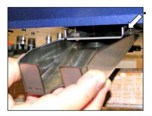
Fix the tag collection tray to the bottom of the machine at the outlet port of the discharge chute.
