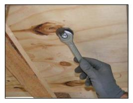
Using a CH 17 wrench remove the clamp nuts of the two anchor pins placed under the pallet top.
