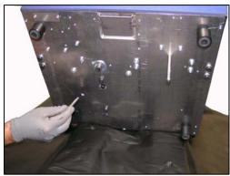
Unscrew the two anchor pins from the base of the machine.
