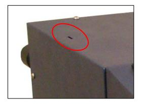
Place the unused loader in the proper slot for storing, on the left side of the embosser cover.
