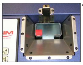
The position of the loader is held in place by a magnet.
