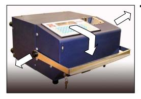
After closing the holes it is possible to lift the machine and place it on a worktop.
