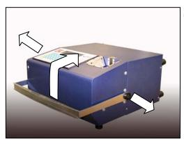
After placing the machine on a worktop lift the handle by pulling the 2 side knobs and move it until it comes close to the top panel.
