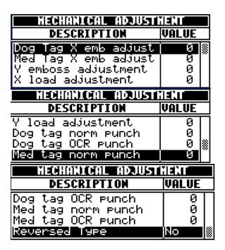
Dog Tag X emb adjust Sets the zero location of the embossing fields with the furthest left edge of the Dog Tag.
