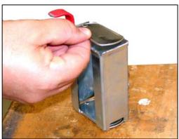
Insert the metal tags with the hanging hole directed towards the left side of the loader and the ridge, only for "DOG TAG" plates. directed upward.
