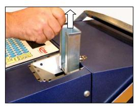
Carefully pull out the tag loader from the machine holding it by the special handle.
