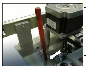
Put the pin in the suitable hole shown by label located on the left side in front of the stepper motor and replace the wing nut.
