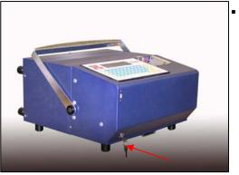
Put the key into the lock, located on the bottom left side of the front panel, and turn it.
