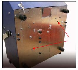
Close the holes of the pins with the M10 screws supplied with the machine.
