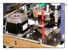
Remove the clamp retainer pin.
